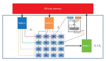
Fig. 2: Diagram of the systolic-array design.
